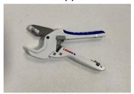
impact and vibration to the LSL when removing from the trench. If necessary, field cut the LSL so that a 5-foot minimum length is available. Cut the pipe with a pipe cutter or pipe shearing device. Do not use a saw. Do not pinch the ends.
